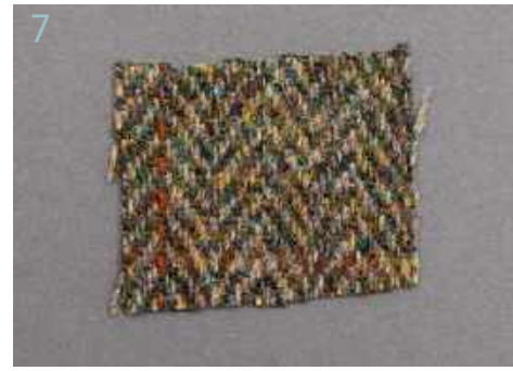
7 INSPECTED AND FINISHED (IT CAN NOW BE CALLED HARRIS TWEED®)
